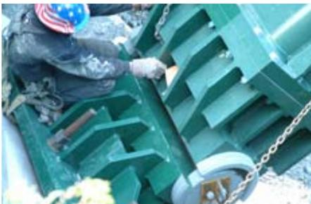
Painted and assembled, the bearing assembly gets a final inspection prior to shipping.
