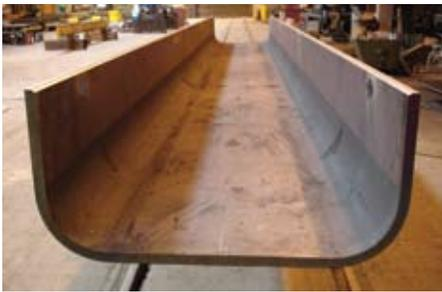
The U-shape was created by cold bending a 1-in. plate. The pieces were then welded together to create a 32-in. x 30-in. rectangular tube.
