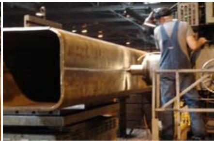
Weld material was removed prior to grinding the weld seams.
