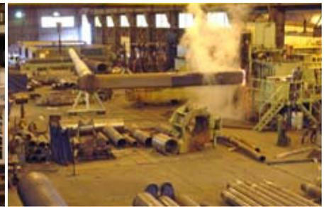
As the tube passes through the induction bender, it is bent to the final radius for each arch.
