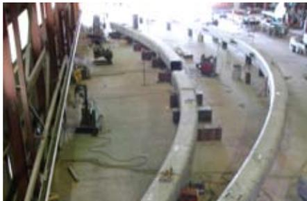
The bent tube sections are fit and welded together to form one of the three segments required for each arch.
