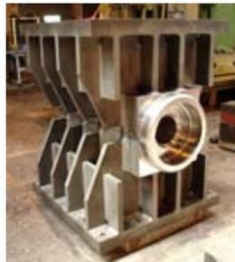
A bearing assembly attaches each end of the arch to the concrete footing. After machining, they are trial fit together.
