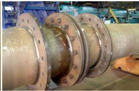
Flanges eliminate the need for field welds.
