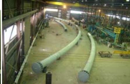
The painted arch segments are ready for shipment.
